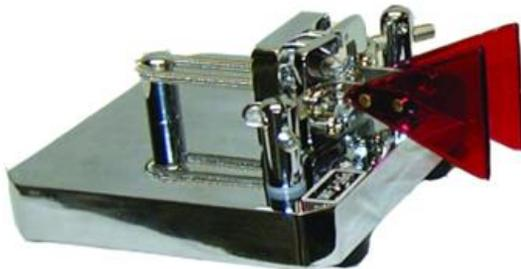
"Iambic" or "squeeze" operation is a feature of the keyer, not the key. With double-lever paddles, both sides can be closed simultaneously by squeezing, hence the name. An electronic keyer set up for iambic or squeeze operation will generate an alternating series of dits and dahs when both paddles are closed at the same time; the series starts with whichever side is closed first. This permits many letters with both dits and dahs to be sent with a single squeeze of the paddles.
