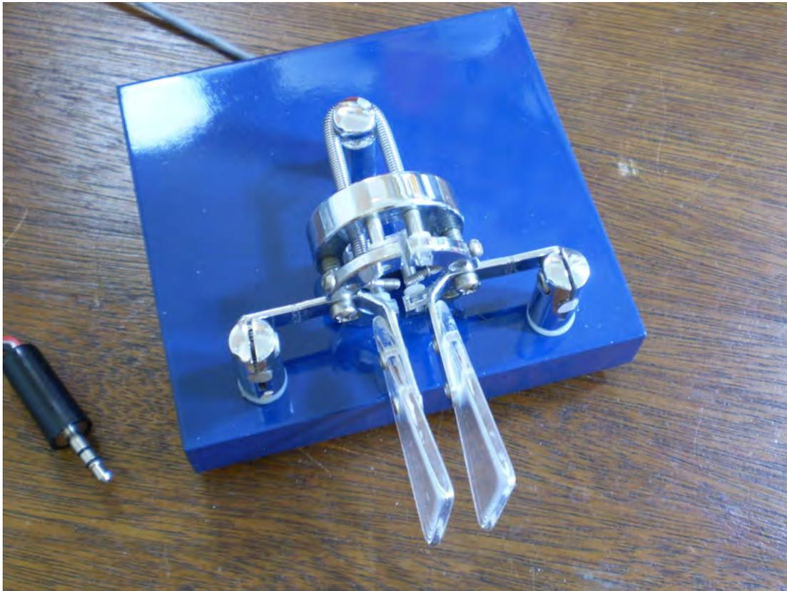
Figure 2: K7QO modifications to a Bencher BY-1.
